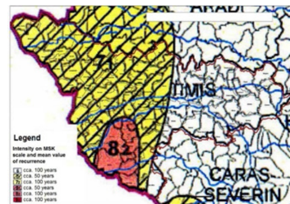
Fig. 3. Intensity on MSK scale and mean recurrence interval
