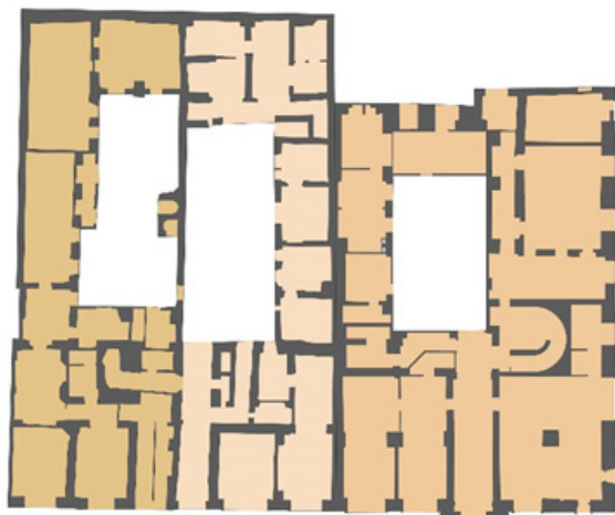
Fig. 2.b) Current plan of the aggregate and distribution of walls and openings at ground floor;
