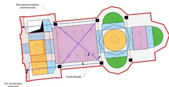
Fig. 5. System of flexible suspension cables
