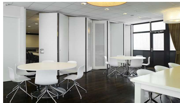
Fig. 13. Foldable mobile walls-"harmonic" type [9]
